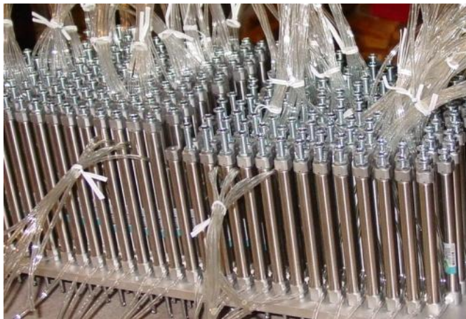
Hook Travel Adjusting Screws and Jam Nuts on TPC Cylinders
